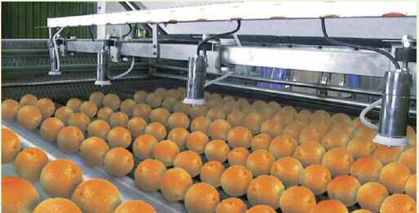
The fine spray unit MAFEX-Potato / MAFEX-Fruit is available with up to four special rotary atomisers. The illustration shows possible application above a sorting table for fruit.
